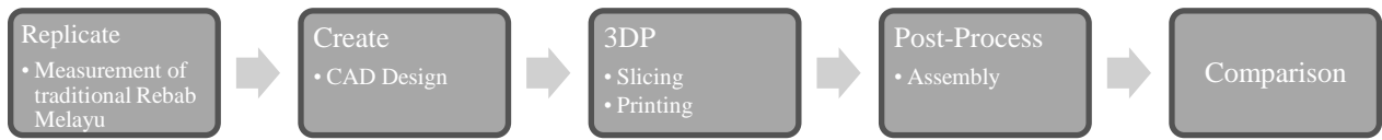
Figure 1. Process of producing 3D-Printed Rebab Melayu adapted from Zoran (2008); Cotrell and Howell (2019)
