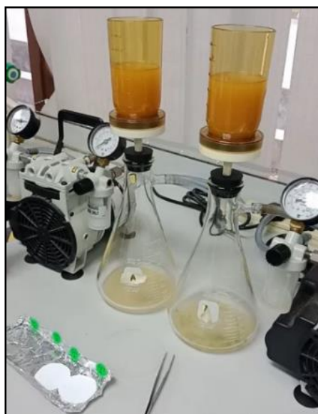
Figure 5. Analysis using vacuum pump filtration and filter paper (Glass Fiber Filter) Suspended sediments that are classified as non-point pollutant are the soil particles formed from the erosion of hills or construction areas that get transported into the river through the surface runoff. According to Gordon et al. (1922), the net weight obtained represents the amount of suspended sediments in the unit of gram per litre.
