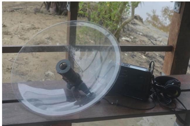
Figure 2. Parabolic Microphone System along with Parabolic Reflector used by the researcher and was described by Wahlström (1985).
