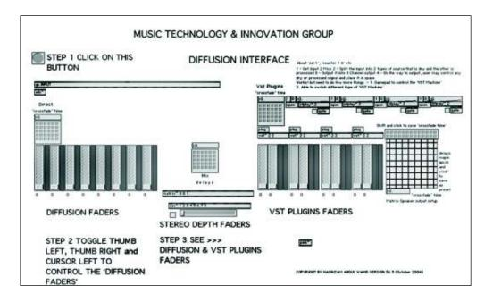
**Figure 3** Example of an 8-channel diffusion interface on Max/MSP with Gamepad as the controller for the faders.
