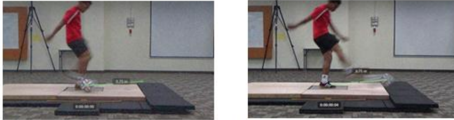
Figure 4: Ball velocity identification using KINOVEA® motion analysis software (free version) during instepkick (original example).
