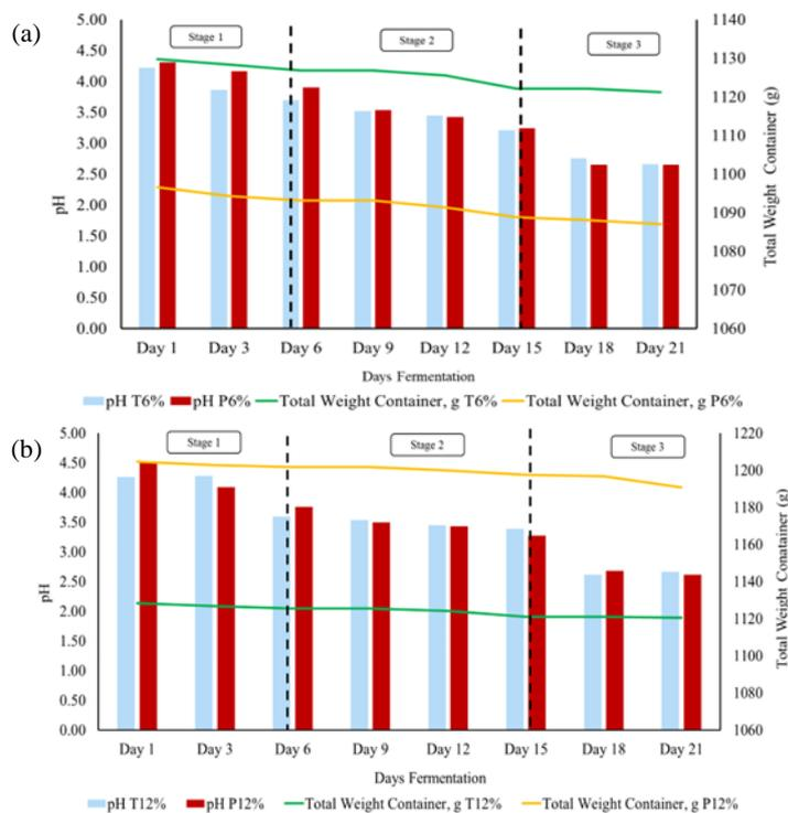
**Figure 3.** Comparison Relationship between pH analysis and Total Weight Container (g) for tea (T) and pumpkin peel (P) wastes as fermentation substrates at (a) 6% (w/v) and (b) 12% (w/v) sugar concentrations.
