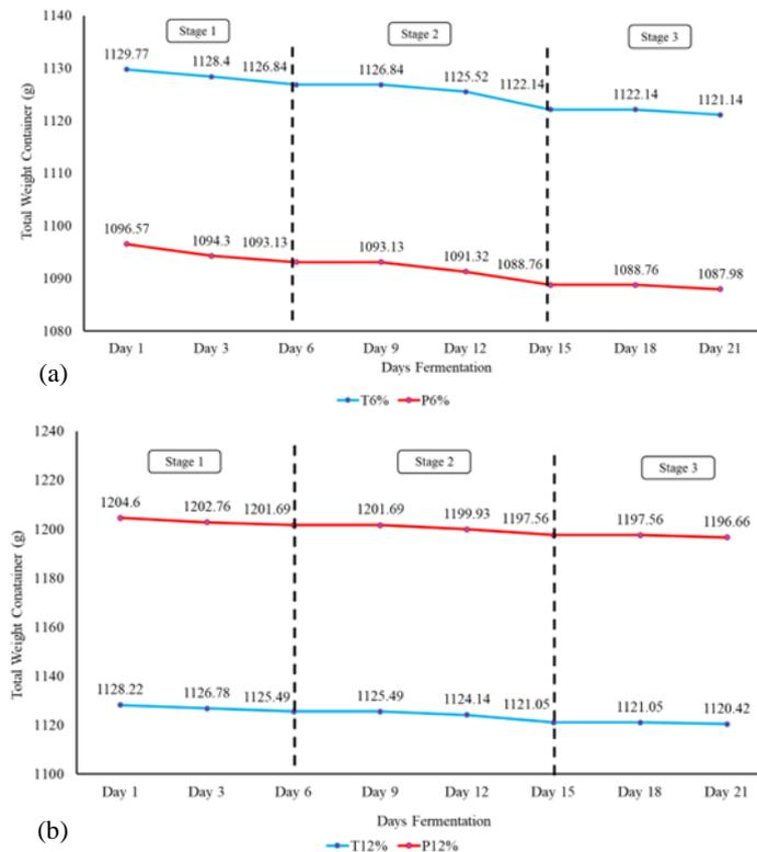
**Figure 2.** Total weight of container (g) during fermentation using tea (T) and pumpkin (P) peel wastes as fermentation substrates at (a), 6% (w/v) and (b) 12% (w/v) sugar concentration.
