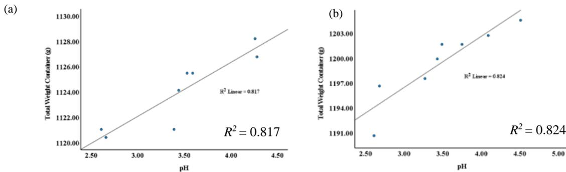
**Figure 5.** Correlation Relationship between pH and Total Weight Container (g/L) for tea (T) and pumpkin (P) peel waste at (a) T12% (w/v) and (b) P12% (w/v) sugar concentration.
