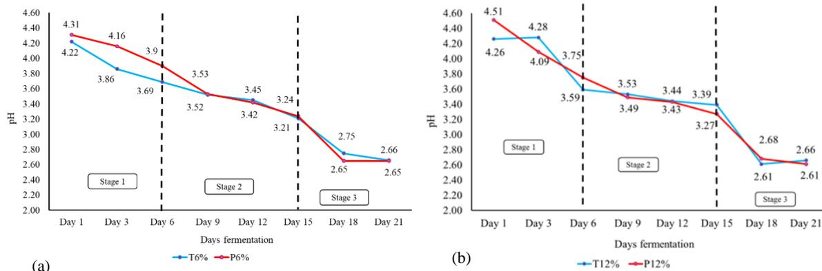
**Figure 1.** pH analysis of fermentation broth using tea (T) and pumpkin (P) peel wastes as fermentation substrates at (a) 6% (w/v) and (b) 12% (w/v) sugar concentrations.
