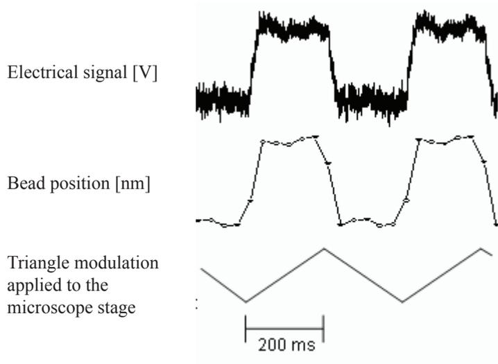
**Figure 3** Responses of the trapped microsphere to a triangular modulation input at the microscope stage position in x-direction.
