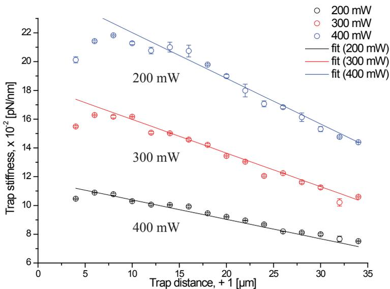
**Figure 7** The trap stiffness independent of the trap distance from the glass surface of the test cell for employed laser power of 200, 300 and 400 mW in PBS at room temperature. The bead diameter is  $2.0 \pm 5\% \mu\text{m}$ .
