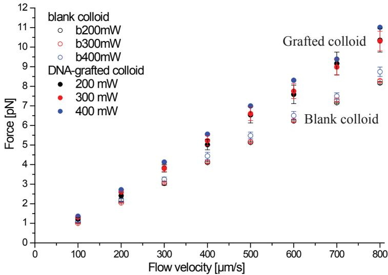
**Figure 6** Representation of **Figure 5** in term of the net force acting on the trapped bead.
