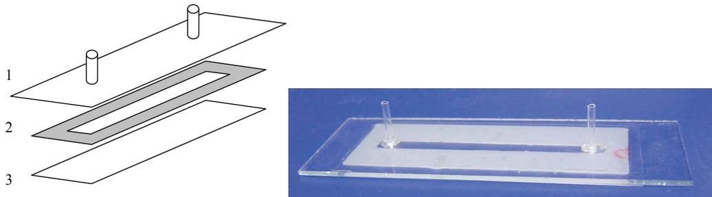
**Figure 2** Left: Test cell construction layers; (1) microscope slide with two capillary tubes attached to it, (2) Parafilm M® layers and (3) cover slide. Right: Test cell real look.
