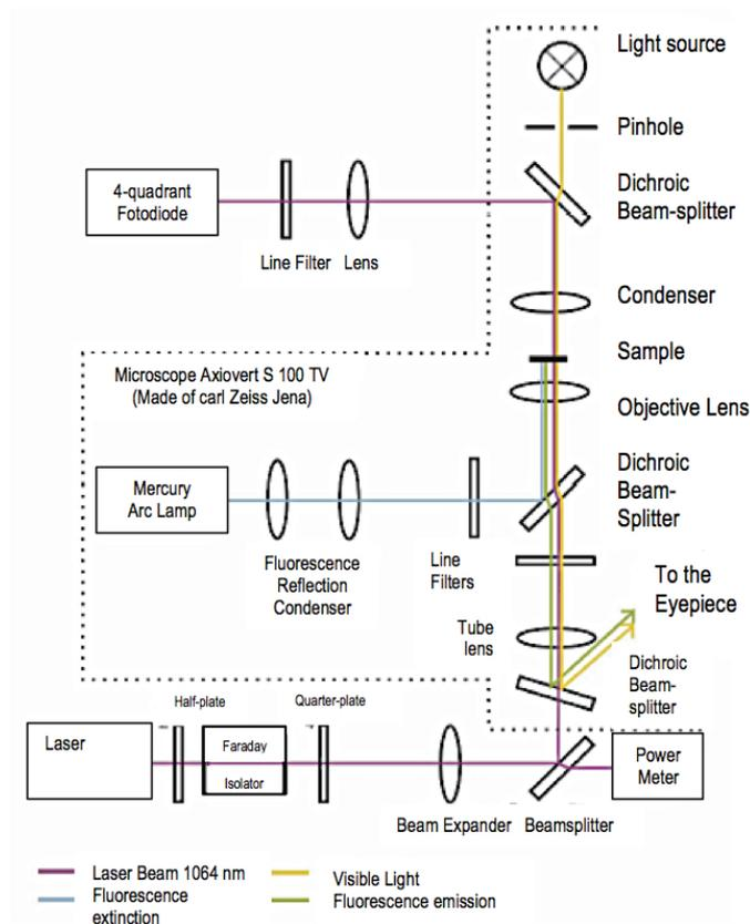
**Figure 1** Optical tweezers setup
