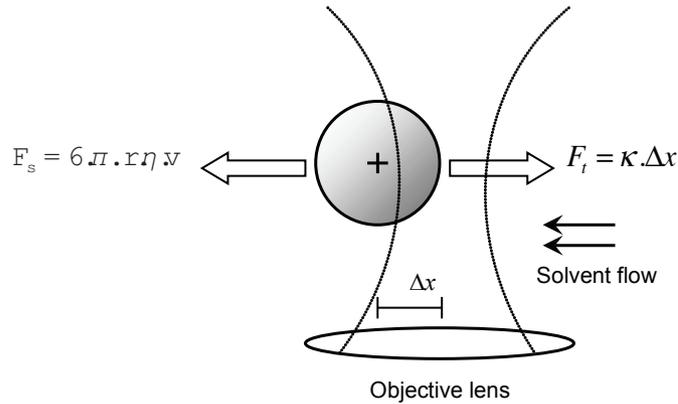
**Figure 4** Illustration on how the trapped bead displaces out of the optical trap centre.
