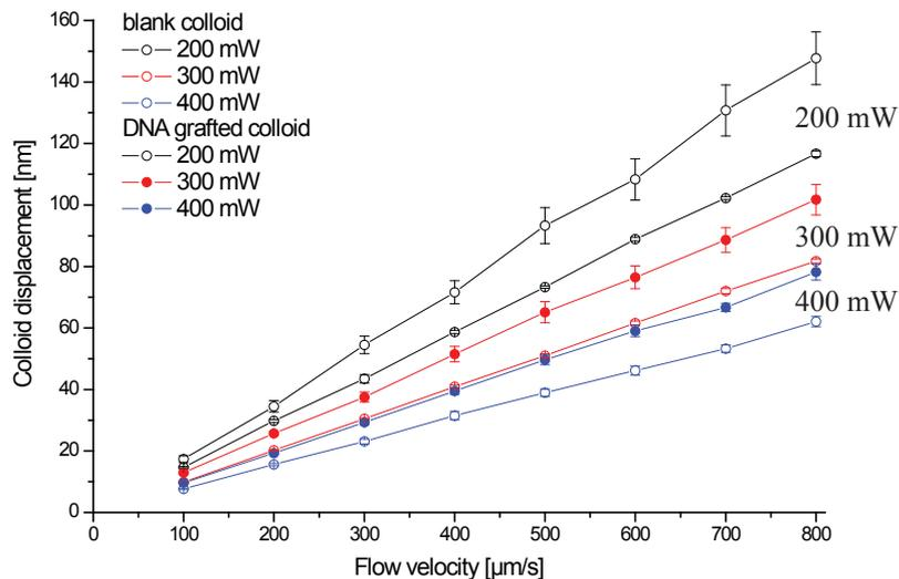
**Figure 5** Displacement of blank and DNA-grafted (4000 bp) polystyrene beads (2.1 μm) in PBS versus flow velocity. The colloid is hold in a distance of 35 μm from the cell ground.
