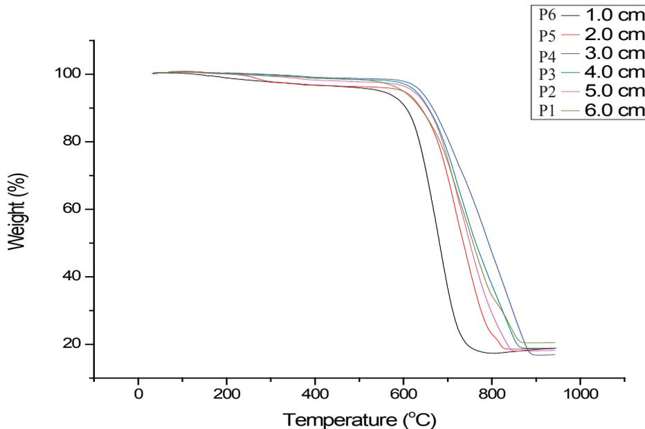
**Figure 4** TGA curves for products synthesized at various location of Si multiple stacking in argon ambient
