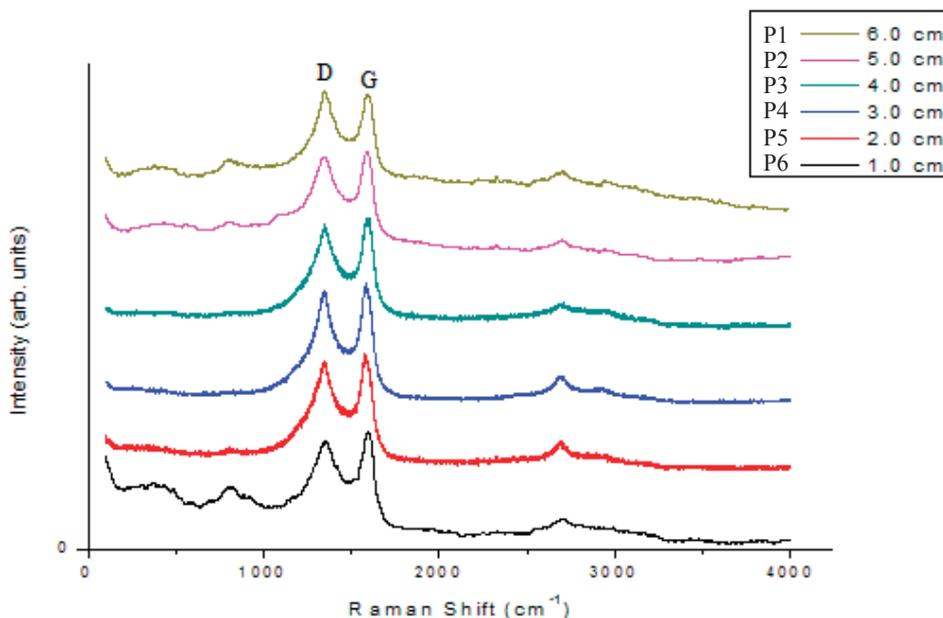
Figure 3 Raman pattern at different substrate position, P1 until P6
