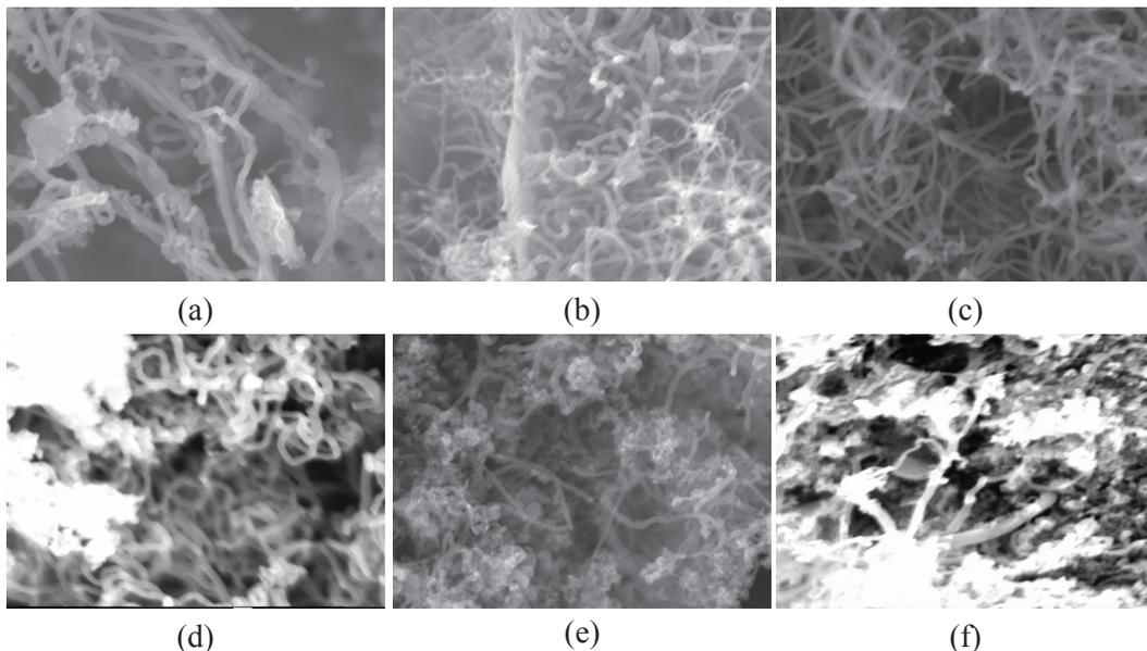
**Figure 2** FESEM images of the CNT synthesized at position: (a) P1, (b) P2, (c) P3, (d) P4, (e) P5 and (f) P6
