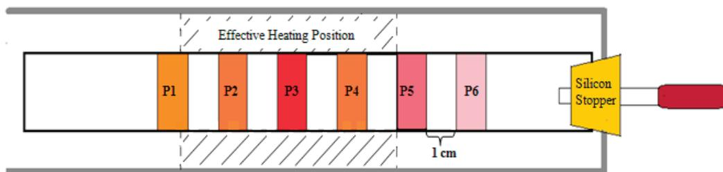
**Figure 1** The schematic diagram of 6 identical substrates positioned on the platform inside the deposition furnace.
