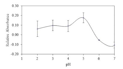
**Figure 3** Effect of solution pH against the reaction of Ferrocenium and 2,4,6-TCP in aqueous solution
