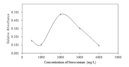
Figure 4 Optimum concentration of ferrocenium against 2,4,6-TCP in aqueous solution.
