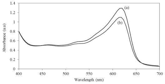
Figure 1 The absorbance spectrum of ferrocenium (a) before and (b) after react with 2,4,6-TCP in aqueous solution
