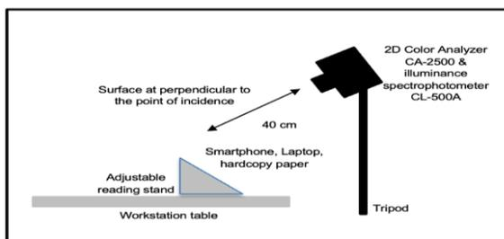
**Figure 1:** Experimental setup of luminance and spectrum profile investigation
