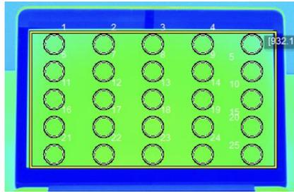
**Figure 2:** The 5 x 5 grid points for measurement of electronic and hardcopy display
