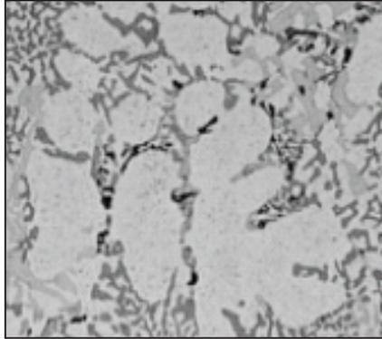
**Figure 1** Microstructure of Mg<sub>2</sub>Si in alloy AA332-F(ASM International, 1992)
