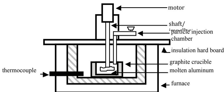
Figure 2 Schematic of stirring mechanism
