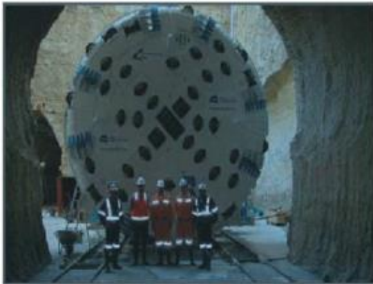
Fig 1.2 Rock Tunnel Boring Machine face, with disc cutters for hard rock Australia [10]
