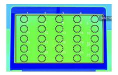
Figure 2: The 5 x 5 grid points for measurement of electronic and hardcopy display
